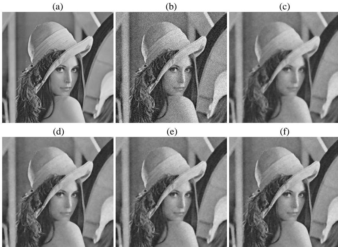
Figure 1. Lenna: (a) The original image, (b) a noisy image contaminated by a Gaussian noise (PSNR=24.8). (c) ~ (f): Restored images from (b) using (c) ITV (d), ABO (e), M-ITV, and (f) M-ABO.
